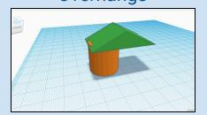
Ordinary 3D printers are not able to print overhangs without support (Details in the **Cura** pamphlet). Try to avoid adding too many overhangs, as supports can decrease the quality of a surface.
